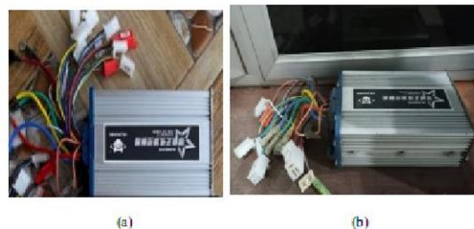
Gambar 2.2 Controller motor listrik (a) 30A (b) 45A
